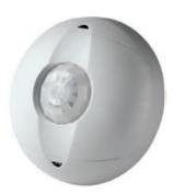
This occupancy sensor mounts quickly to the ceiling and directly connects to KMC Lighting cabinets. The passive infrared sensing features a semiconductor heat detector behind a Fresnel lens. This multi-zone lens establishes dozens of areas of detection. The sensor is sensitive to the heat emitted by the human body. The sensor triggers only when the source of heat moves from one zone of sensing to another. Hot stationary objects and air currents do not cause false triggers. Other features include
