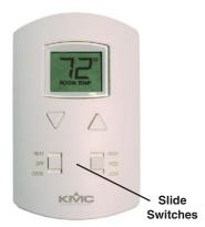
This is a wall-mounted, temperature-sensing, programmable operator interface for use in a KMC direct digital controls system. It includes intuitive-to-use setpoint buttons, and two **slide switches for heating/cooling change over and fan speed**. (Humidity is not sensed or displayed, and it does not have a hinged cover.) Four-pin EIA-485 (formerly RS-485) data port on the underside for easy temporary computer connection to the controller.
